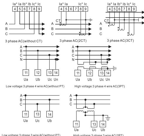
Note: The meter is provided with two kinds of wiring modes, please make sure the actual wiring is same to the set wiring in the meter. The wiring diagram and technical parameter printed on the product shall be prevailed.
